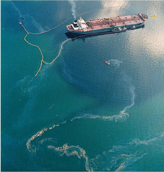
A floating containment barrier (or boom) encircles the Exxon oil tanker *Valdez* after its grounding on a reef off the coast of Alaska. Exxon was found negligent in the environmental disaster and was ordered to pay \$5.3 billion for the cleanup. On appeal, the company managed to reduce the damages to \$500 million based on academic research that it had funded—research that some scholars believe involved a conflict of interest.
