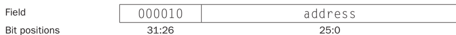
FIGURE 4.23 Instruction format for the jump instruction (opcode = 2). The destination address for a jump instruction is formed by concatenating the upper 4 bits of the current PC + 4 to the 26-bit address field in the jump instruction and adding 00 as the 2 low-order bits.
