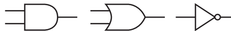
FIGURE B.2.1 Standard drawing for an AND gate, OR gate, and an inverter, shown from left to right. The signals to the left of each symbol are the inputs, while the output appears on the right. The AND and OR gates both have two inputs. Inverters have a single input.
