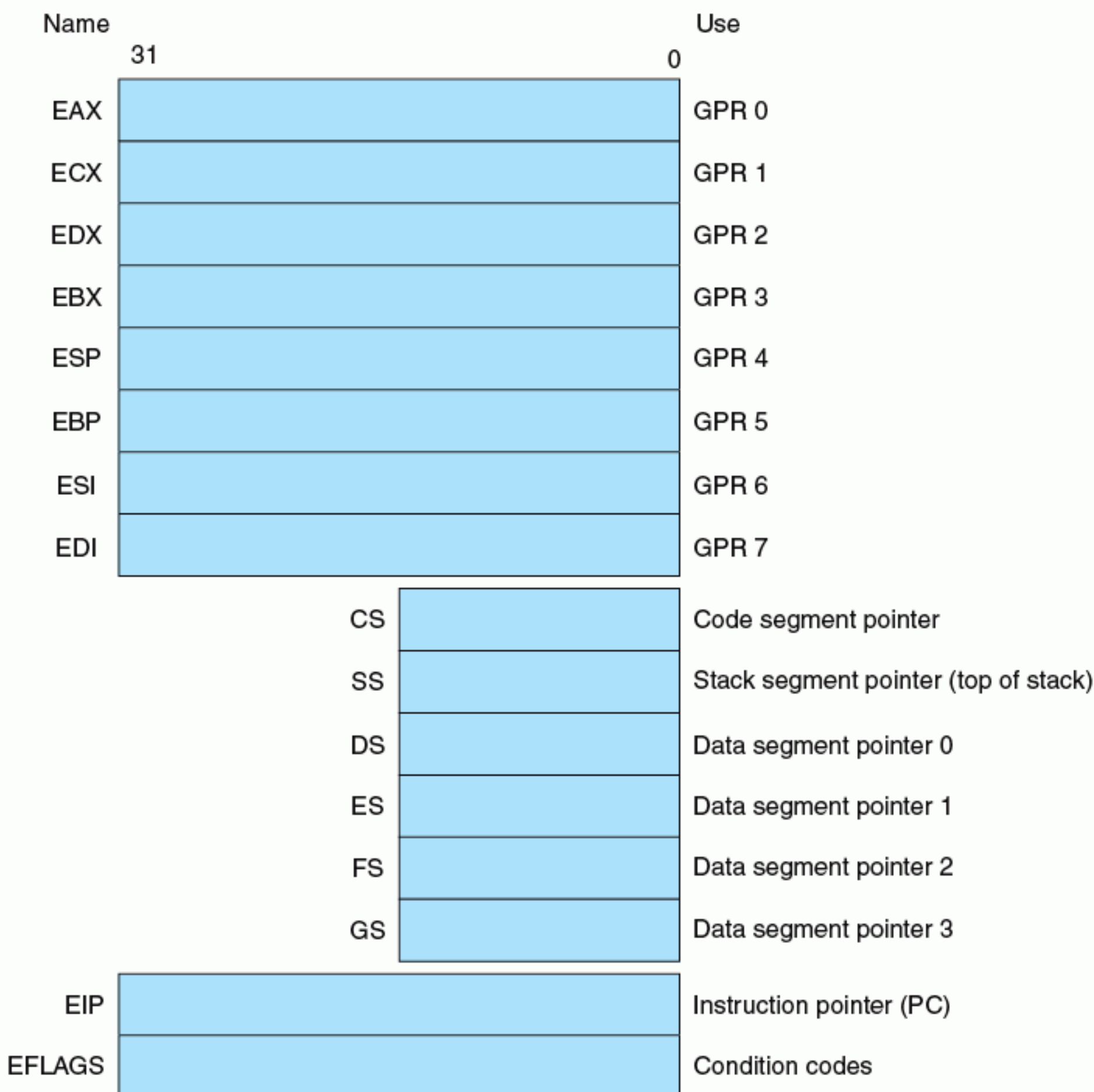
FIGURE 2.40 The 80386 register set. Starting with the 80386, the top eight registers were extended to 32 bits and could also be used as general-purpose registers.
