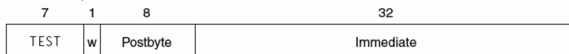
FIGURE 2.45 Typical IA-32 instruction formats. Figure 2.46 shows the encoding of the postbyte. Many instructions contain the 1-bit field w , which says whether the operation is a byte or double word. The d field in MOV is used in instructions that may move to or from memory and shows the direction of the move. The ADD instruction requires 32 bits for the immediate field because in 32-bit mode the immediates are either 8 bits or 32 bits. The immediate field in the TEST is 32 bits long because there is no 8-bit immediate for test in 32-bit mode. Overall, instructions may vary from 1 to 17 bytes in length. The long length comes from extra 1-byte prefixes, having both a 4-byte immediate and a 4-byte displacement address, using an opcode of 2 bytes, and using the scaled index mode specifier, which adds another byte.
