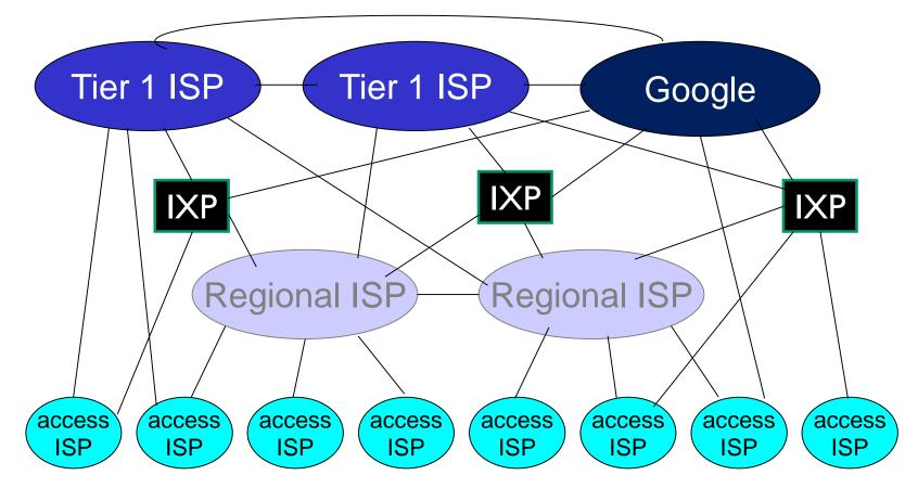
at center: small # of well-connected large networks
