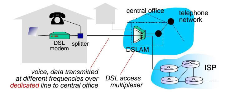
suse existing telephone line to central office DSLAM
