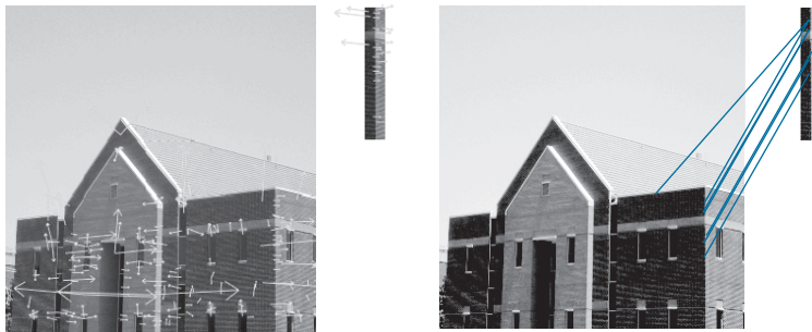
FIGURE 11.65 (a) Keypoints for the half-sized building and a section of the right corner. (b) Corresponding keypoints between the corner and the building. Of the seven matches found, only one is in error.
