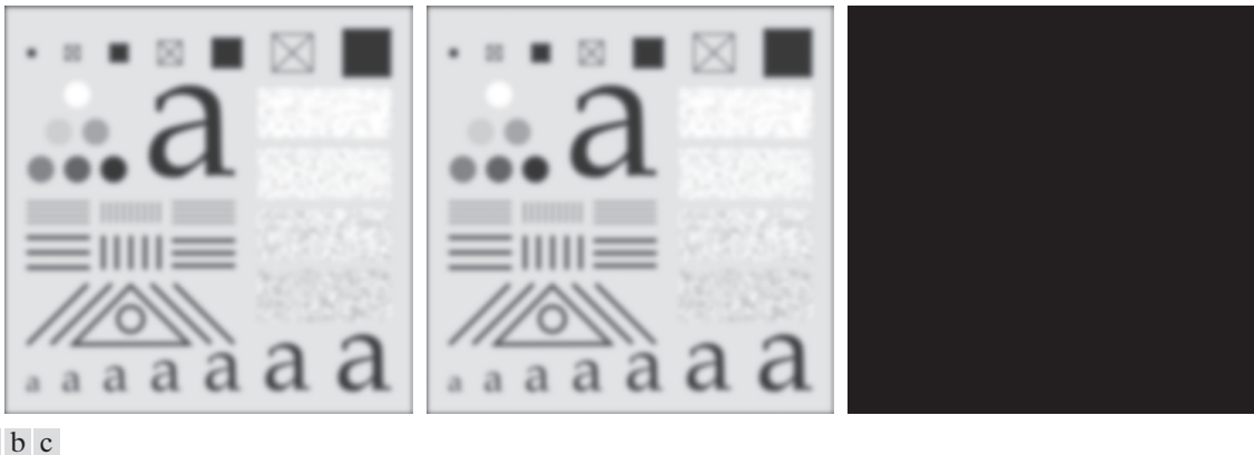
FIGURE 3.37 (a) Result of filtering Fig. 3.36(a) using a Gaussian kernels of size 43 \times 43 , with \sigma = 7 . (b) Result of using a kernel of 85 \times 85 , with the same value of \sigma . (c) Difference image.
