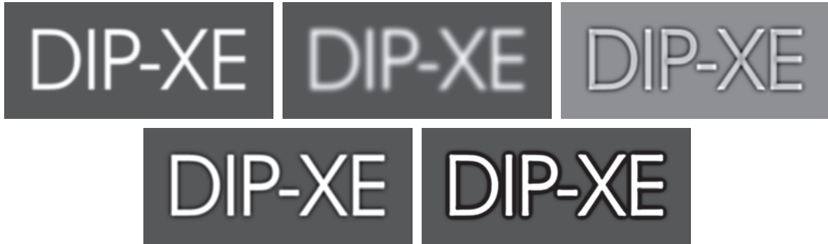
FIGURE 3.49 (a) Original image of size 600 \times 259 pixels. (b) Image blurred using a 31 \times 31 Gaussian lowpass filter with \sigma = 5 . (c) Mask. (d) Result of unsharp masking using Eq. (3-56) with k = 1 . (e) Result of highboost filtering with k = 4.5 .
