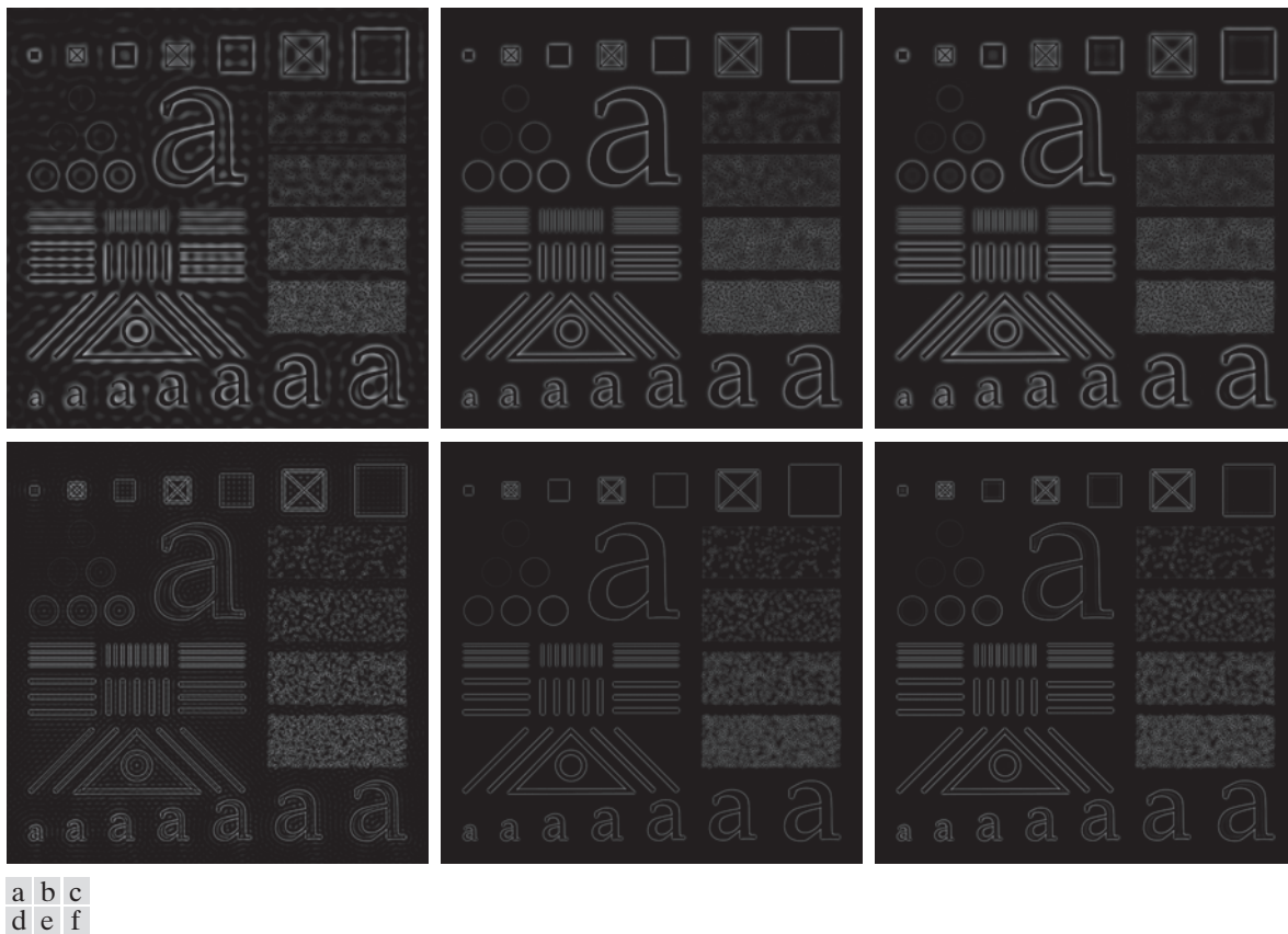
FIGURE 4.53 Top row: The image from Fig. 4.40(a) filtered with IHPF, GHPF, and BHPF transfer functions using D_0 = 60 in all cases ( n = 2 for the BHPF). Second row: Same sequence, but using D_0 = 160 .
