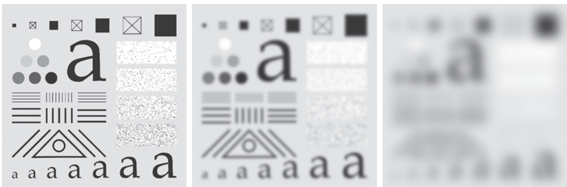
FIGURE 3.40 (a) Test pattern of size 4096 \times 4096 pixels. (b) Result of filtering the test pattern with the same Gaussian kernel used in Fig. 3.39. (c) Result of filtering the pattern using a Gaussian kernel of size 745 \times 745 elements, with K = 1 and \sigma = 124 . Mirror padding was used throughout.
