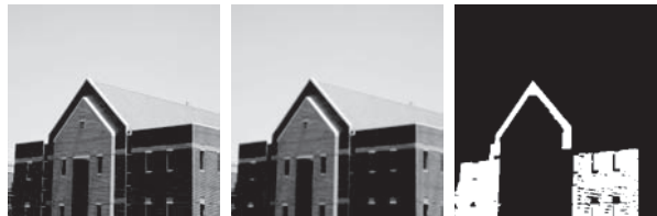
FIGURE 11.55 (a) Building image reduced to half-size. (b) Image smoothed with a 3 \times 3 box kernel. (c) Composite MSER obtained with the same parameters as Fig. 11.53(e), but using a valid MSER region size range of 2,500–7,500 pixels.
