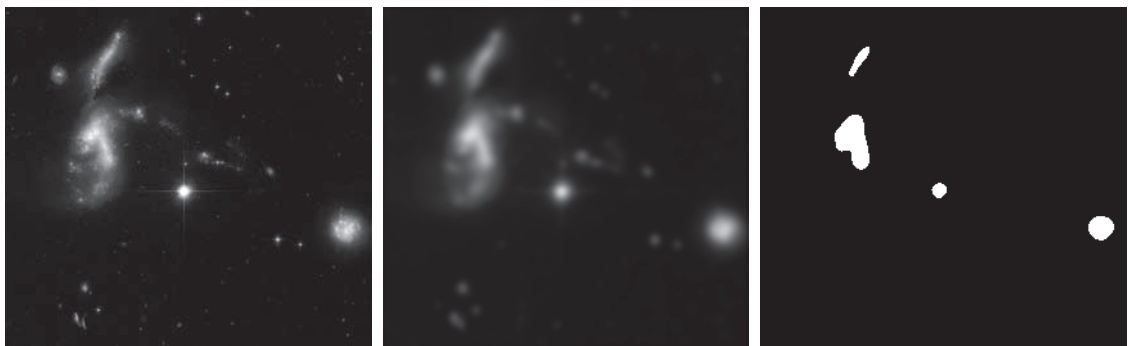
FIGURE 3.41 (a) A 2566 \times 2758 Hubble Telescope image of the Hickson Compact Group . (b) Result of lowpass filtering with a Gaussian kernel. (c) Result of thresholding the filtered image (intensities were scaled to the range [0, 1] ). The Hickson Compact Group contains dwarf galaxies that have come together, setting off thousands of new star clusters. (Original image courtesy of NASA.)
