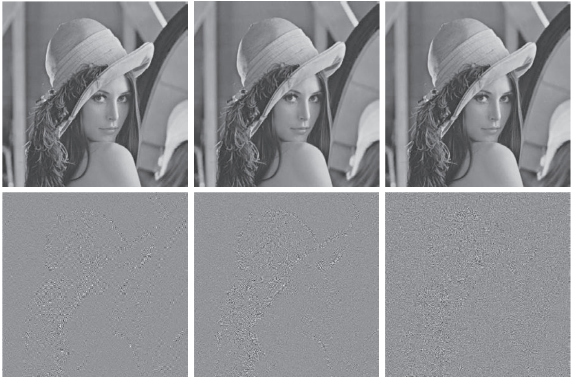
FIGURE 8.22 Approximations of Fig. 8.9(a) using the (a) Fourier, (b) Walsh-Hadamard, and (c) cosine transforms, together with the corresponding scaled error images in (d)–(f).
