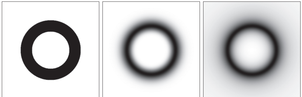
FIGURE 4.63 (a) The ideal, (b) Gaussian, and (c) Butterworth bandpass transfer functions from Fig. 4.62, shown as images. (The thin border lines are not part of the image data.)
