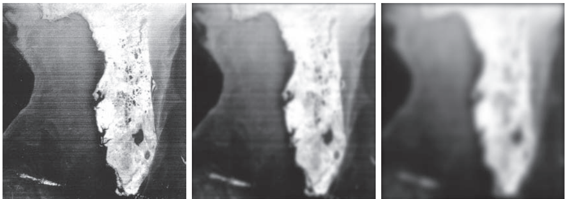
FIGURE 4.50 (a) 808 \times 754 satellite image showing prominent horizontal scan lines. (b) Result of filtering using a GLPF with D_0 = 50 . (c) Result of using a GLPF with D_0 = 20 . (Original image courtesy of NOAA.)
