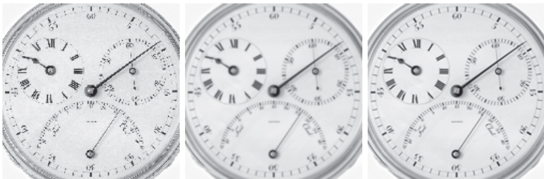
FIGURE 2.27 (a) Image reduced to 72 dpi and zoomed back to its original 930 dpi using nearest neighbor interpolation. This figure is the same as Fig. 2.23(d). (b) Image reduced to 72 dpi and zoomed using bilinear interpolation. (c) Same as (b) but using bicubic interpolation.
