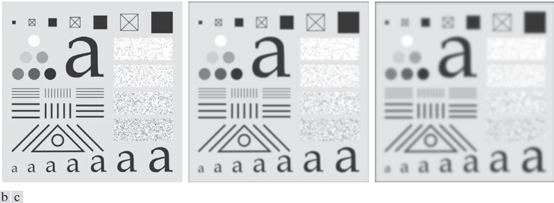
FIGURE 3.36 (a) A test pattern of size 1024 \times 1024 . (b) Result of lowpass filtering the pattern with a Gaussian kernel of size 21 \times 21 , with standard deviations \sigma = 3.5 . (c) Result of using a kernel of size 43 \times 43 , with \sigma = 7 . This result is comparable to Fig. 3.33(d). We used K = 1 in all cases.
