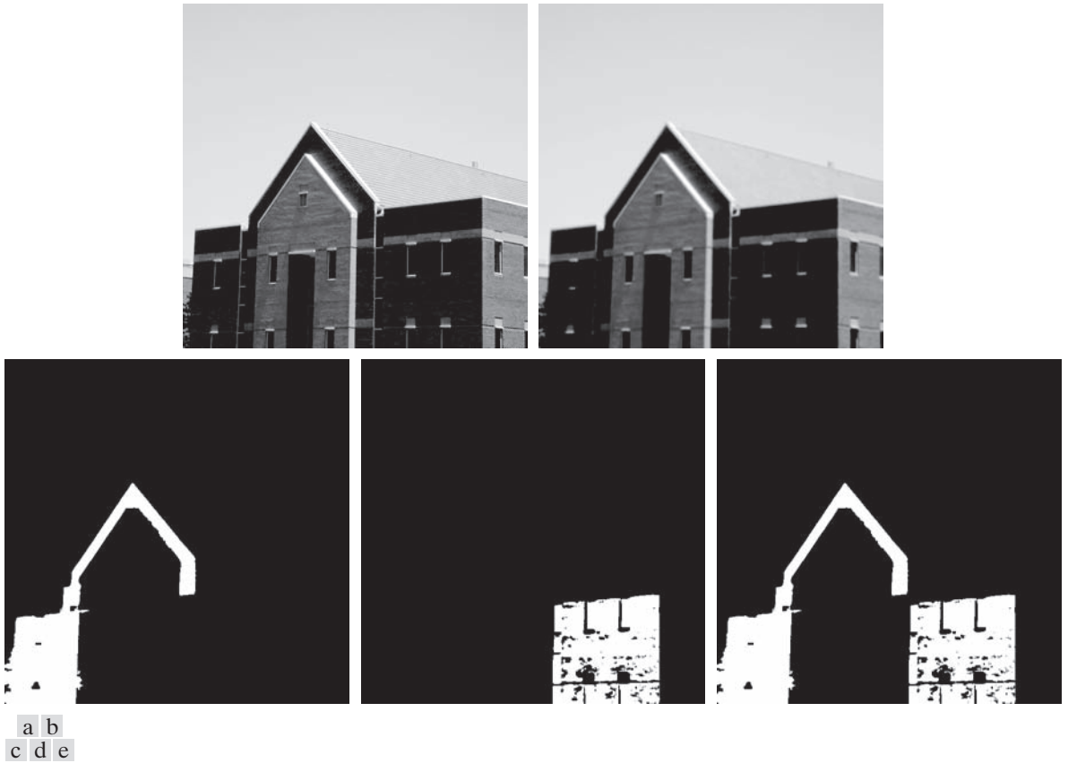
FIGURE 11.53 (a) Building image of size 600 \times 600 pixels. (b) Image smoothed using a 5 \times 5 box kernel. (c) and (d) MSERs detected using T = 0 , \Delta T = 10 , and MSER size range between 10,000 and 30,000 pixels, corresponding approximately to 3% and 8% of the area of the image. (e) Composite image.
