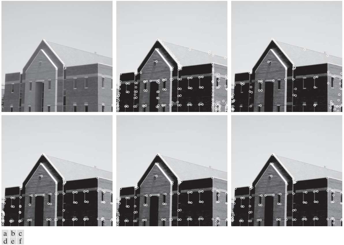
FIGURE 11.49 600 \times 600 image of a building. (b) Result of applying the HS corner detector with k = 0.04 and T = 0.01 (the default values in our implementation). Numerous irrelevant corners were detected. (c) Result using k = 0.249 and the default value for T . (d) Result using k = 0.17 and T = 0.05 . (e) Result using the default value for k and T = 0.05 . (f) Result using the default value of k and T = 0.07 .
