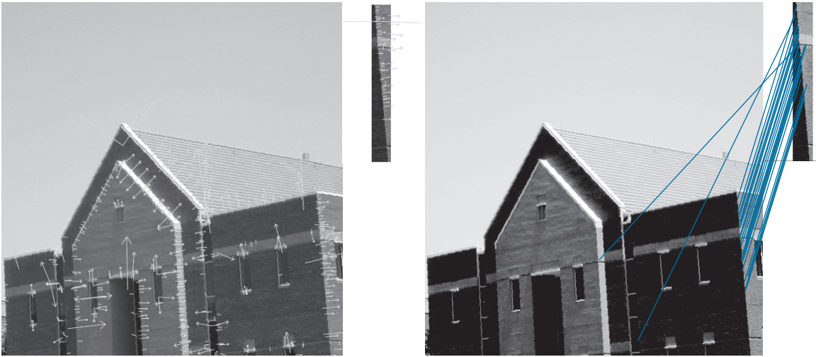
FIGURE 11.64 (a) Keypoints for the rotated (by 5^\circ ) building image and for a section of the right corner of the building. The subimage is a separate image and was processed as such. (b) Corresponding keypoints between the corner and the building. Of the 26 matches found, only two are in error.
