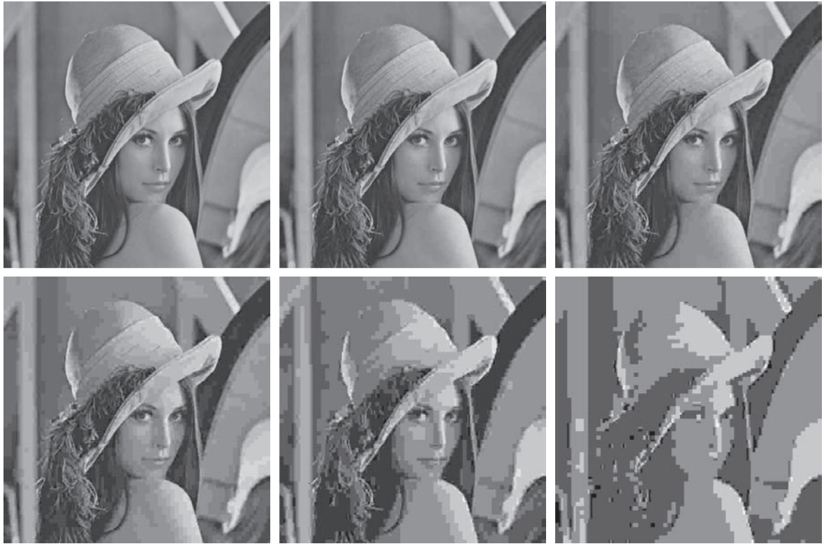
FIGURE 8.28 Approximations of Fig. 8.9(a) using the DCT and normalization array of Fig. 8.27(b): (a) Z , (b) 2Z , (c) 4Z , (d) 8Z , (e) 16Z , and (f) 32Z .
