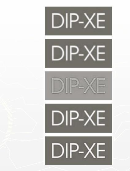
b d FIGURE 3.40 (a) Original image. (b) Result of blurring with a Gaussian filter. (c) Unsharp mask. (d) Result of using unsharp masking. (e) Result of using highboost filtering.
