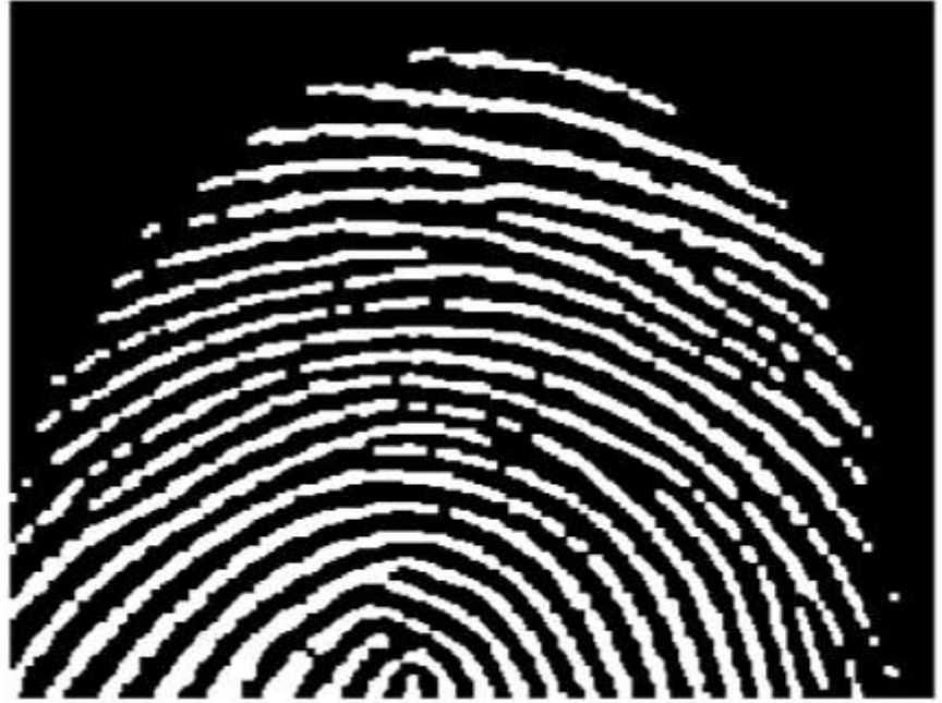
Image after segmentation and morphological processing
