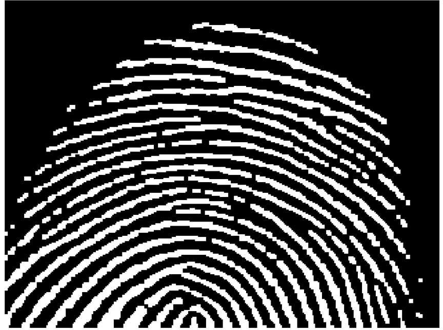
Image after segmentation and morphological processing
