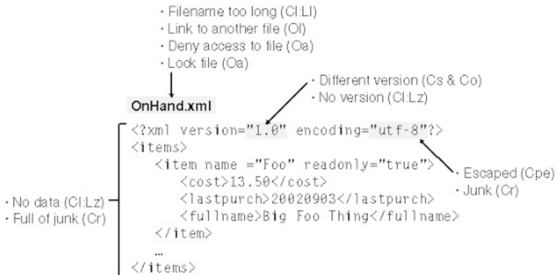
Figure 19-2. Examples of mutating some XML elements, including the filename.
