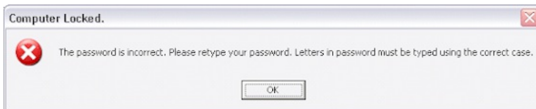
Figure 24-3. An example of a good error message, with no information disclosure errors.
