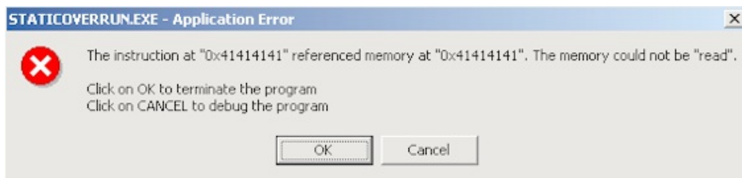
Figure 5-1. Application error message generated after the stack-based buffer overrun occurs.
